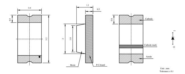
Electrodes: Au Plating Encapsulating Resin: Epoxy Resin Package: BT Resin
